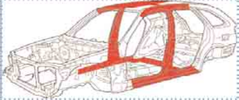
The Mazda 323's triple-H body construction gives strength where it's needed most – around the passenger cell.
